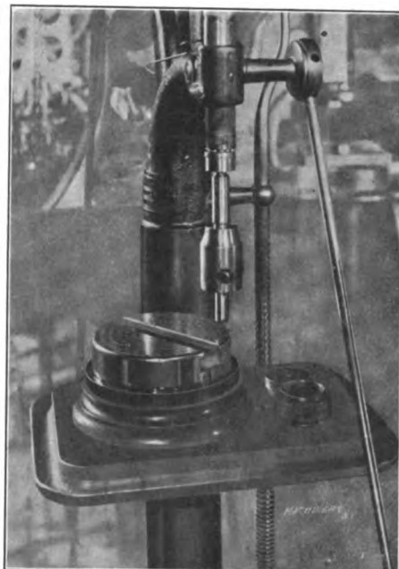
Fig. 17. Damaskeening the Turntable Top in a Drill Press
