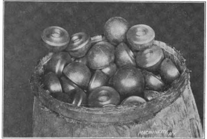
Fig. 2. Partly finished Castings for the Spherical Base
