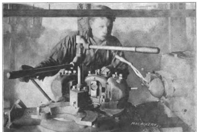
Fig. 4. Centering the Spherical Base
